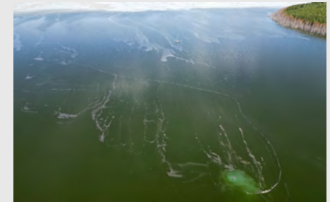
Nitrogen gas bubbles in the Gibraltar TSF indicating the in-situ process is working
