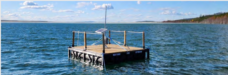
Monitoring barges installed in the Gibraltar TSF collecting real-time water quality data
